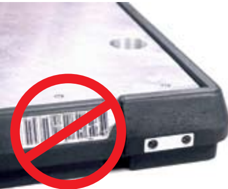
Bar codes are not reliable on assembly pallets.
